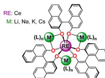
Figure 1. Shibasaki's REMB framework. RE = rare earths; M = Li, Na, K; B = (S)-BINOLate; RE/M/B = 1:3:3.
